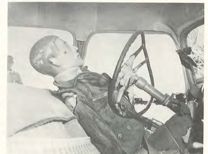
The result of crashing an automobile at 30 mph into a brick wall. The dummy, instrumented to determine the shocks on a human being, is pinned between the seat and the broken steering wheel. In addition to improving crash protection for aircraft, such studies at HADC will pave the way for safer automobiles.
